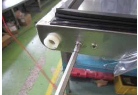
G. Assemble stopper plate in original positions.
