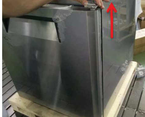
2) Remove the top hinge from the unit.
